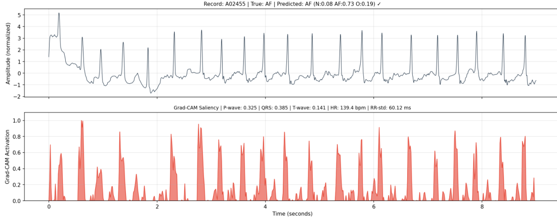
Figure 3: Example Grad-CAM saliency map for a correctly classified AFib sample. Top: raw ECG signal. Bottom: Grad-CAM activation along the same time axis, with peaks indicating regions the model focused on.
